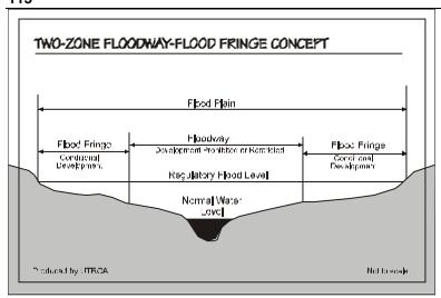
**Flood Fringe** is defined as the outer portion of the floodplain between the floodway and the flooding hazard limit. Depth and velocities of flooding are generally less severe in the flood fringe than those experienced in the floodway. The flood fringe is the area where development or site alteration may be permitted, subject to appropriate flood proofing to the flooding hazard elevation or other flooding hazard standard approved by the Ministry of Natural Resources.
