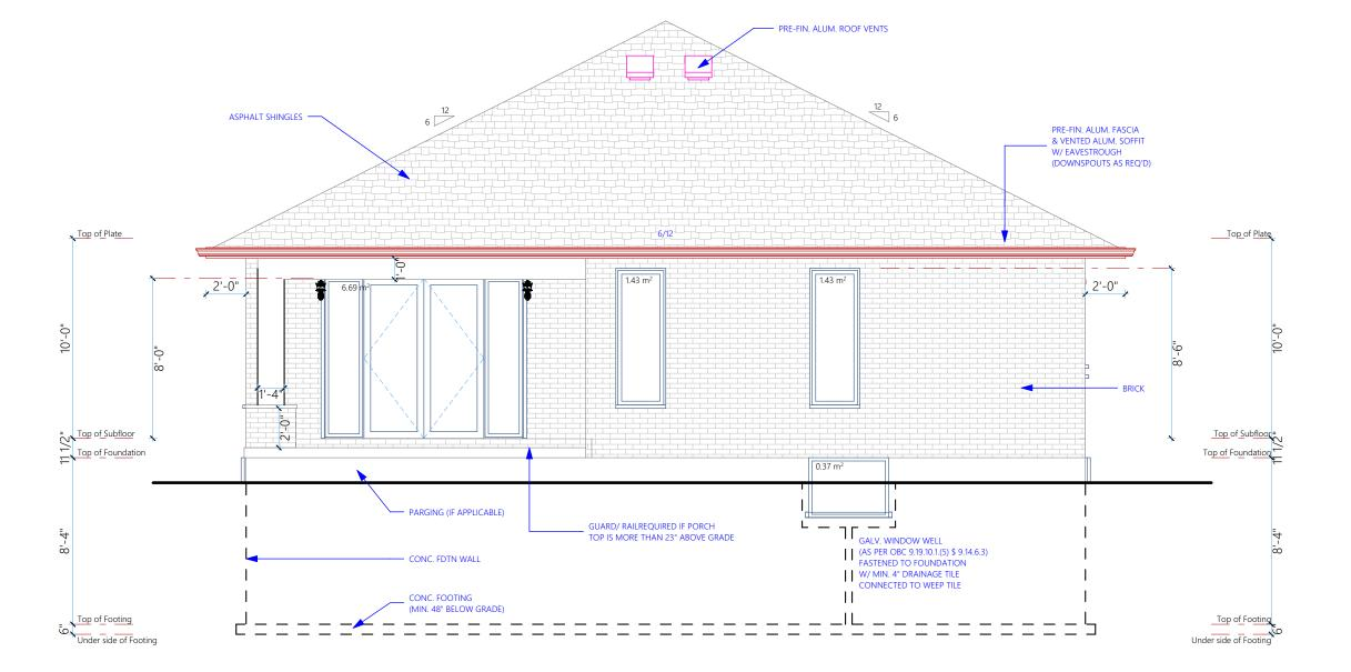
DO NOT SCALE DRAWINGS. WORK TO DIMENSIONS SHOWN. THE CONTRACTOR MUST CHECK ALL DRAWINGS AND VERIFY ALL DIMENSIONS ON THE JOB. ALL STEEL ANGLES SUPPORTING BRICK VENEER TO HAVE MIN. 6" BEARING @ ENDS, TYP.
