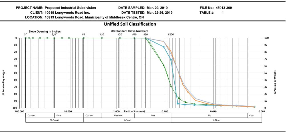
Description Symbol Borehole ID Sample # Sample Depth MW101-19 0.76-1.37 mbgs Silty SAND, trace Clay SS-2 -CERTIFIED BY MW102-19 0.76-1.37 mbgs -SS-2 Sandy SILT, trace Clay MW102-19 4.57-5.18 mbgs SILT, some Sand, trace Clay SS-6 MW103-19 4.57-5.03 mbgs SS-6 Sandy SILT, trace Clay Canadian Council of Independent Laboratories
